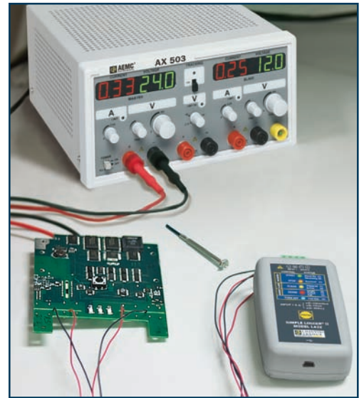
L432 recording two DC voltage supplies.
