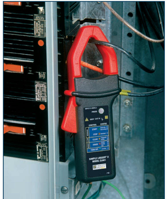
Easily log current in power panels.
