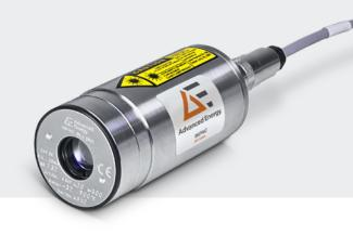
The Impac<sup>®</sup> IN 5 plus series infrared thermometers are specially designed for non-contact temperature measurements on non-metallic surfaces and also on painted, coated or anodized metals. These instruments are digital pyrometers equipped with a digital interface, enabling temperature indication and storage on a PC. A temperature sub range can be also configured and the instrument parameters can be adjusted remotely.
