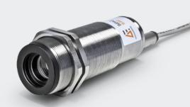
The Impac® IS 210 and IGA 210 are stationary pyrometers for non-contact temperature measurement of metal surfaces, graphite, ceramics etc. The digital pyrometers use the two-wire format that combines the high accuracy of the digital signal processing with the simple connection and operation with two wires.
