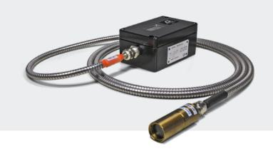
The Impac® ISR 50-LO digital, highly is an accurate two-color pyrometer with fiber optic for non-contact temperature measurements in temperature ranges between 700 and 3000°C. The instrument is equipped with an optical fiber, which can be used in very high ambient temperatures up to 250°C without cooling and it is unaffected by electromagnetic interferences.
