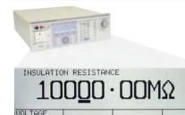
Continuously variable Insulation resistance to 2GOhms @ 1000V. A high accuracy option (0.1%) is available to support the new generation of higher accuracy insulation testers.
