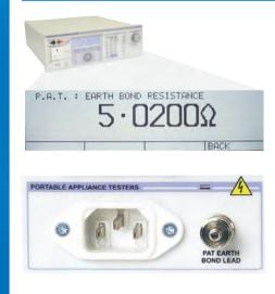
The 3200 provides easy connection for earth bond resistance tests using a front panel mounted 'floating' earth stud. The 3200 is supplied with a calibrated PAT lead to connect to the PAT mains socket for the best accuracy.
