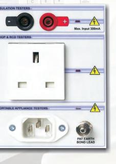
Dedicated mains sockets for Loop, RCD & PATs on the 3200 front panel avoids the need to make connection of mains voltages/power using 4mm type test leads. This important safety feature eliminates any risk of shock to the engineer as connections are made with standard mains type plugs.
