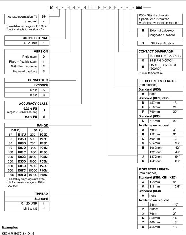
Melt pressure transducer with type "J" thermocouple,4...20mA output, 6-pin connector, 1/2-20UNF thread, 00 bar pressure range, 0.5% accuracy class, 153 mm (6") rigid stem, 457mm (18") flexible stem, Inconel 718 diaphragm, SIL2 certification.
