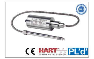
The HWE series of Gefran are pressure transmitters with HART communication protocol for using in high temperature environment. The main characteristic of this series is the capability to read temperature of the media up to 315°C. The constructive principle is based on the hydraulic trasmission of the pressure.
