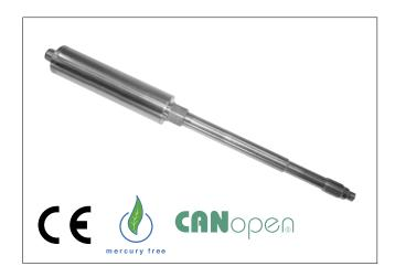
The KD Series are for use in high temperature applications where the process temperatures may reach 538°C (1000°F) such as high temperature engineered polymers. The K Series utilizes standard melt pressure principles and construction, but uses a near incompressible NAK (Sodium Potassium) for pressure transmission. The K Series strain sensing technology is thick film on Stainless Steel.
