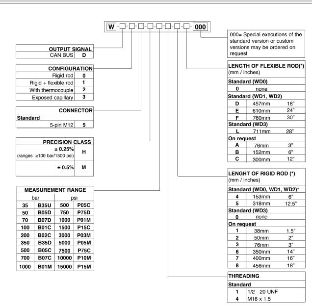
(\*) note: max. total length of rigid/flexible rod is 914 mm-36"
