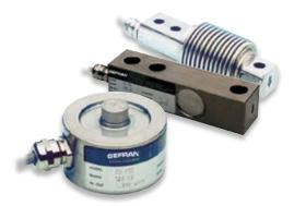
Load cells and force transducers are used in many industrial applications. They have an electrical output in mV/V and a measurement range from 50 Kg to 50,000 Kg.
