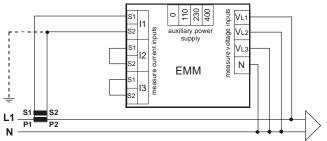
N.B. If the multimeters are used on single phase line, the measure are referred on the L1 phase. The others datadisplayed relatives at three phase system are not to consider.
