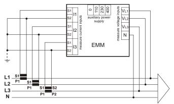
N.B. on line with 3 wires (without neutral or with neutral not supplied) the N terminaln must not be connected.
