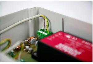
Do not forget to tighten the cable glands to ensure a waterproof installation.
