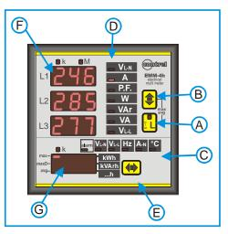
The integration for the calculating of the average values is synchronized all the time that the instrument turn on. Press **A** and **B** keys another time to come back to the measures visualization. The instrument will come back to the measure visualization automatically if for 10 seconds no one button is pressed.
