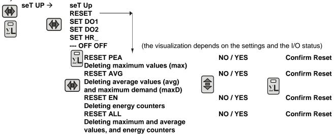
To enable the chosen type, press the **B** key to change the indication on display **G** from **NO** to **yes**.
