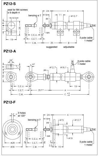
Important: all the data reported in the catalogue linearity, lifetime, temperature coefficient are valid for a sensor utilization as a ratiometric device with a max current across the cursor lc  $\leq$  0.1  $\mu$ A.
