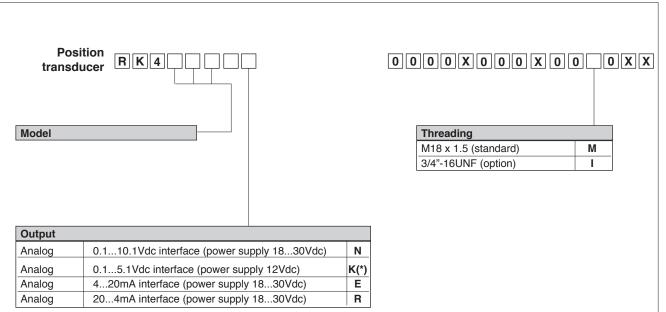
(\*) The maximum stroke for the K version is 1200mm
