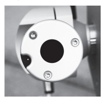
**RaZON**<sup>+</sup> is an innovative ALL-IN-ONE solar monitoring system with integrated pyrheliometer, shaded pyranometer, digital data processing, GPS receiver and data logger. It measures DNI from the sun and DHI from the sky and, knowing the sun position, calculates GHI that matches secondary standard value. From the DNI measurements sunshine duration is calculated much more accurately than any sunshine duration sensor on the market.
