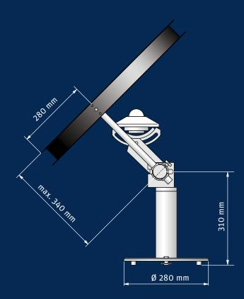
The ring has a width / diameter ratio of 0.185 and has a view of 10.6° seen from the radiometer. Because the ring intersects a part of the diffuse sky, a table is supplied to compensate the measured values.
