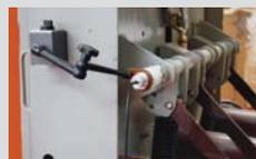
**PME-ATA:** Angular measurement set consisting of digital angular encoder, 19-mm machineable shaft adapter bushing, and articulated arm with magnetic stand.
