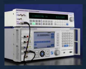
For calibration of high accuracy frequency counters, a 1ppm high stability frequency output is available (Included in 4010)
