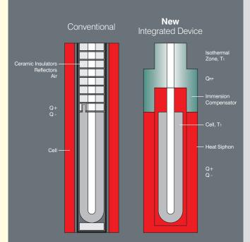
A fixed point cell is not long enough to eliminate heat conductance along the thermometer calibrated in it.
