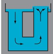
Here the heating, cooling and mixing take place in one of two parallel tubes. The second tube is the calibration volume and again the excellent temperature uniformity gives small calibration uncertainties
