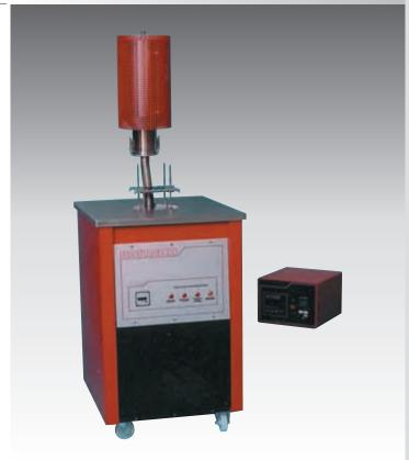
A disadvantage of many fluidized-bed baths is that good temperature stability and uniformity cannot be achieved in the fluidized medium itself. They are obtained by using large metal blocks or by inhibiting the fluidizing action in the powder around the work piece - either locally, or by completely collapsing the bed at the required temperature, this is not the case with the 875. A full evaluation report is available upon request.
