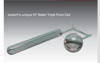
Reverting to the very first designs of water triple point cells, Isotech produce a cell with Isotopic analysis, a McLeod gauge to assess any trapped air and an attached flask where the cell's water can be transferred and redistilled. By accounting for these sources of uncertainty we claim that this cell represents the ultimate reference for those requiring cells as close to ITS-90 as possible. Please ask for a copy of a comprehensive report describing the cell, its operation and performance.
