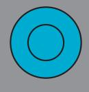
In this design liquid is forced down an outer tube and flows up an inner concentric tube. The heating and cooling takes place in the outer tube leaving the inner tube as the calibration volume into which the thermometers are immersed. This design gives very small vertical and axial temperature gradients
