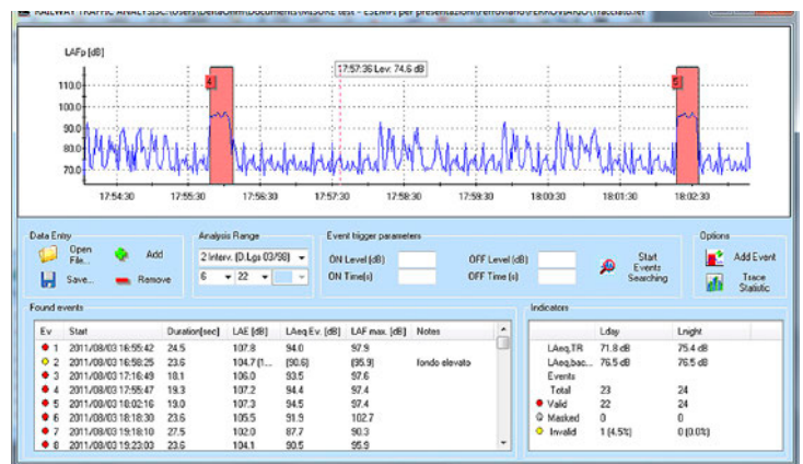
Noise Studio: NS2A "Acoustic Pollution" module; railway traffic noise, 24h analysis with automatic identification of train transits.
