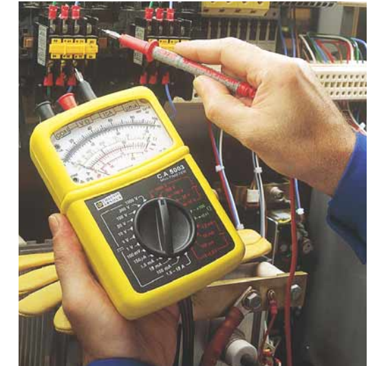
▲ Voltage test with the C.A 5003. The black test prod is in the "hands free" position, held in the multi-purpose clip on the back of the instrument.
